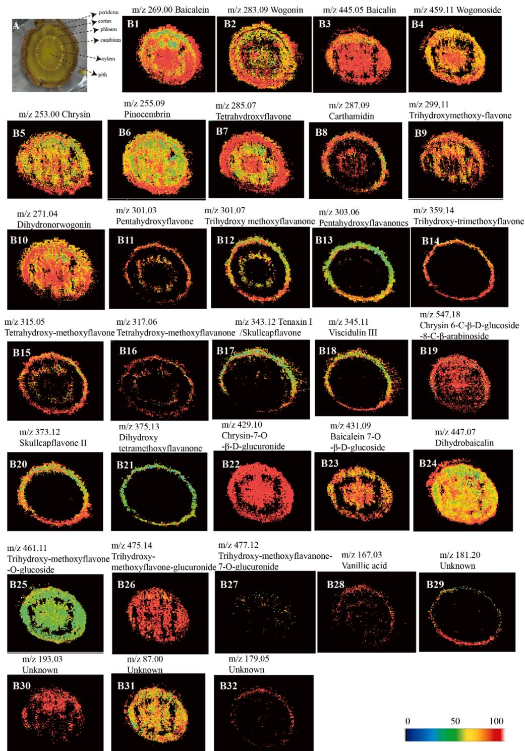
**Fig 2.** (A) Optical image of the root section (B) MS images of representative metabolites in *Scutellaria baicalensis* root sections. Color scales encode arbitrary ion relative strength.
