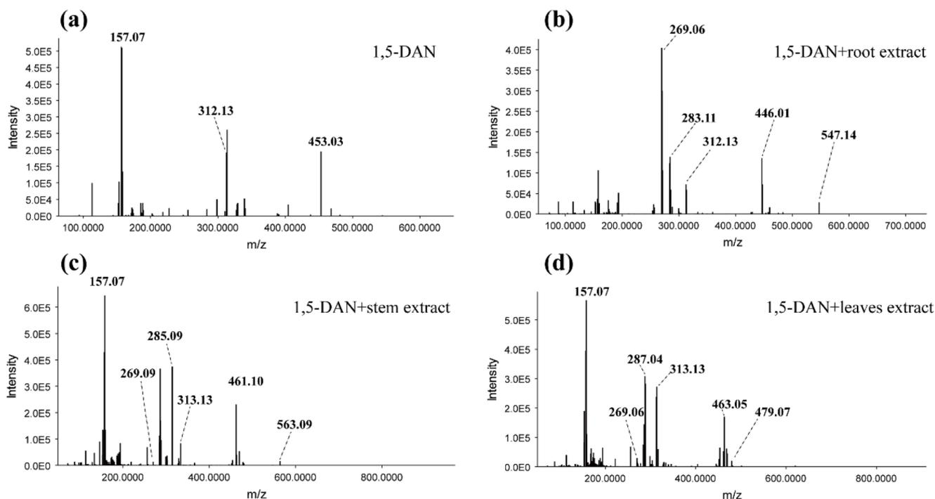
**Fig. 1.** MALDI-TOF MS spectra of *Scutellaria baicalensis* extracts analyzed in negative ion mode by using 1,5-DAN (a) 1,5-DAN (b) 1,5-DAN + root extract, (c) 1,5-DAN + stem extract (d) 1,5-DAN + leaves extract.
